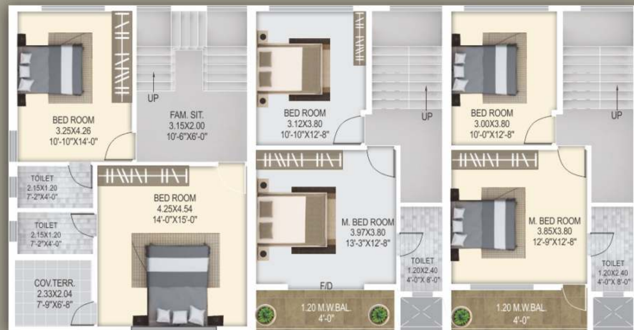
SECOND FLOOR PLAN
