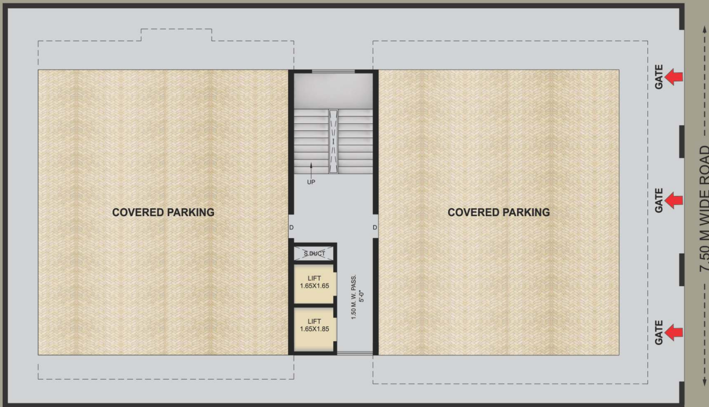
PARKING FLOOR PLAN ( 'E' TYPE, P+7 )
