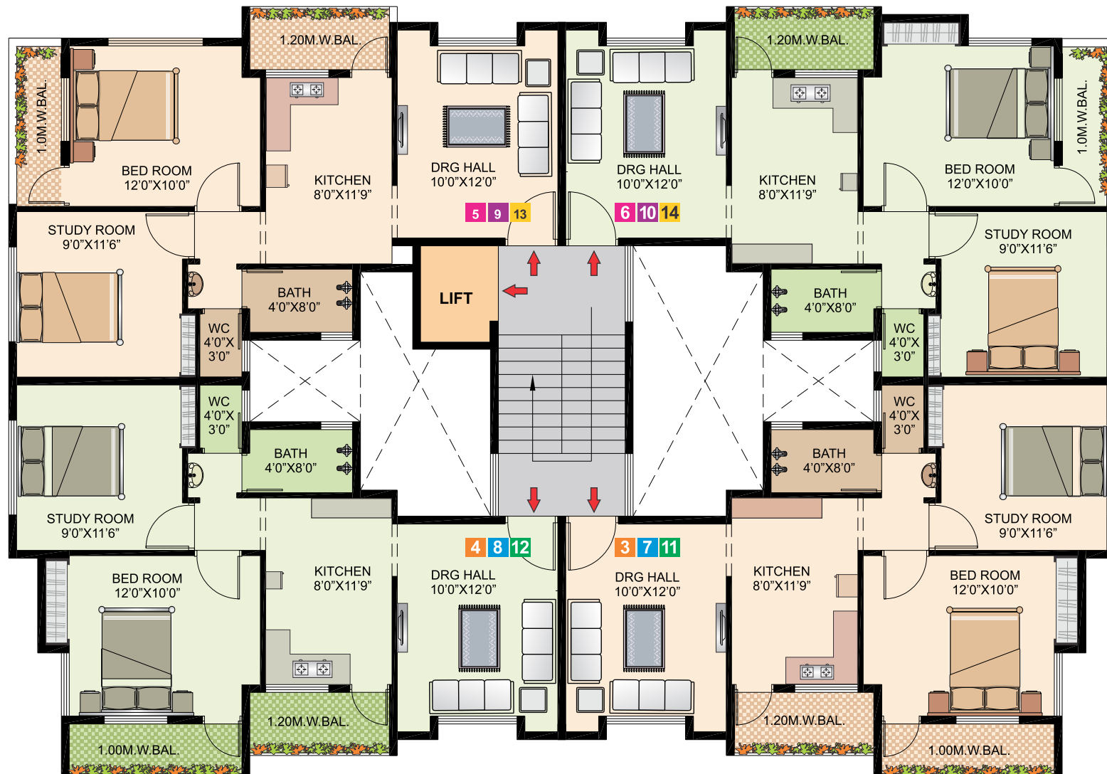
STILT, FIRST, STILT FIRST SECOND, STILT SECOND, THIRD FLOOR PLAN
