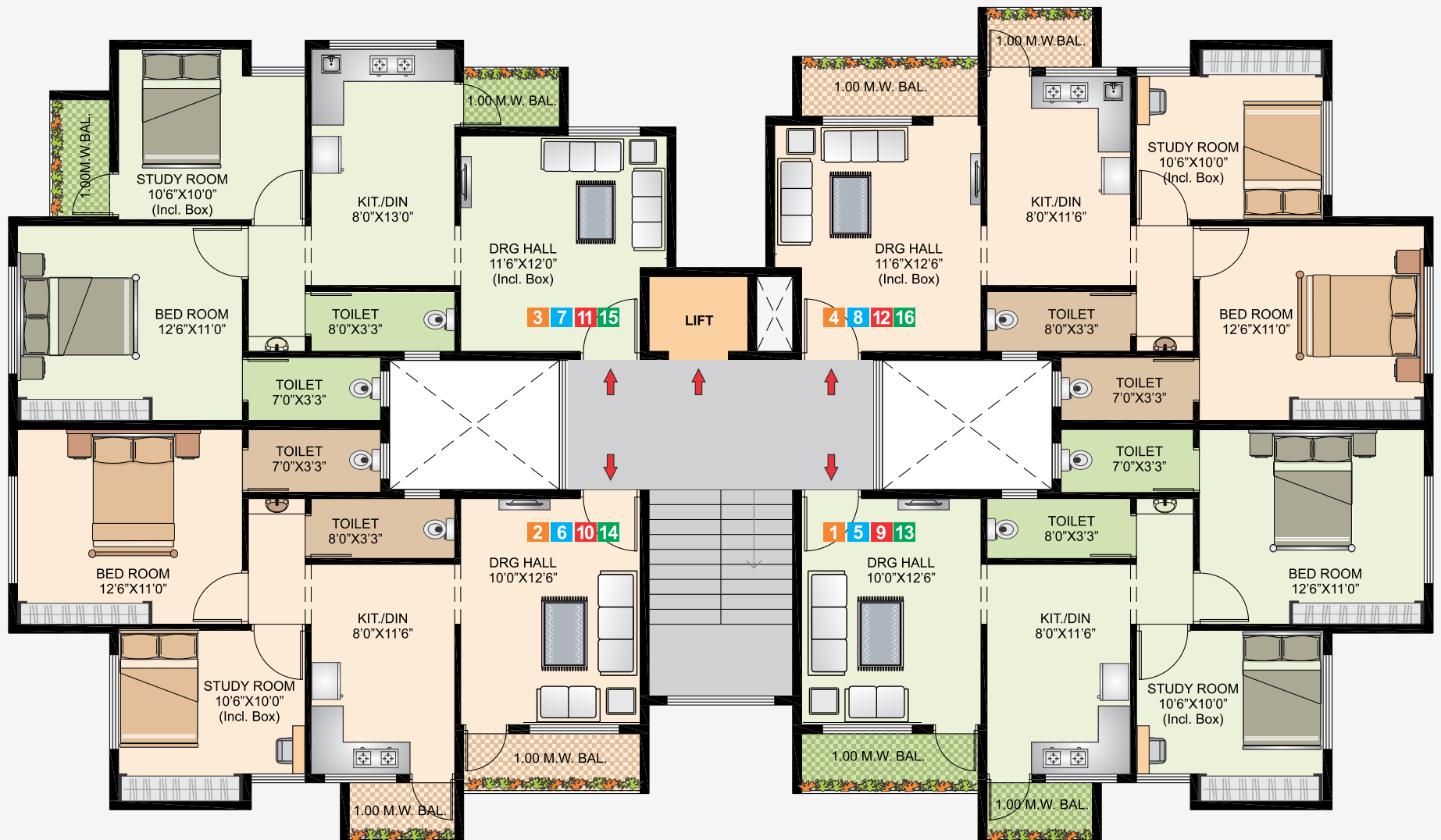
TYPICAL STILT, STILT FIRST, STILT SECOND, STILT THIRD FLOOR PLAN
